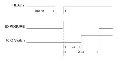
Figure 53. Timing for Experiment Setup shown in Figure 52
